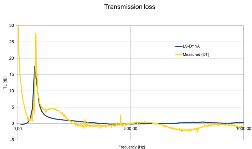
Fig. 7: Comparison between experimental and simulated transmission loss data for a certain configuration of Helmholtz resonator.
