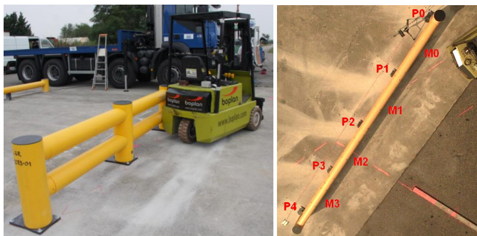
Fig. 1: Test set-up (left) and impact point designation (right)
