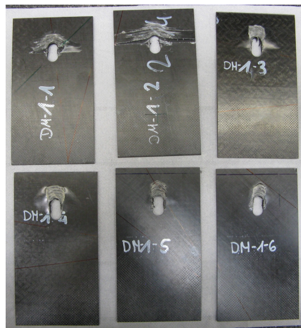
Fig. 15: Failure pattern of the bearing test specimen.
