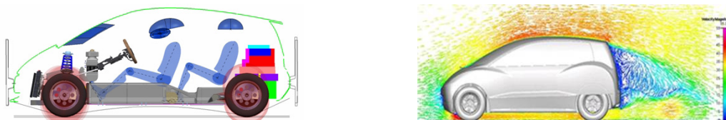
Figure 3: BEV packaging theme and aerodynamic study
