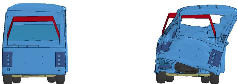
Figure 11(a): New bus condition after rollover Figure 11(b): Aged bus condition after rollover
