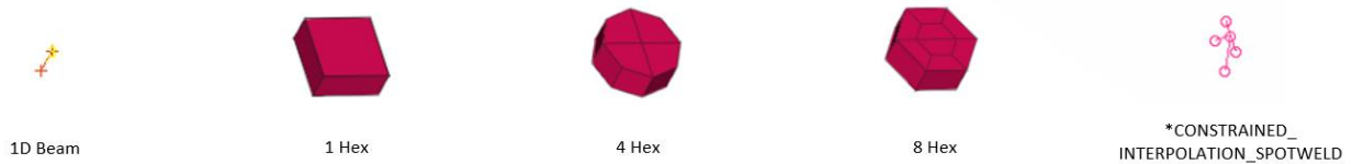
Fig.2: Different types of weld representation in LS-Dyna
