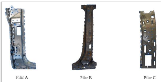
Fig.3: Pillars A, B and C from Chevrolet Silverado 2014. Images taken from A2MAC1 platform.
