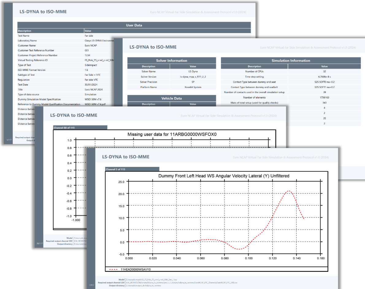
Fig.14: LS-DYNA to ISO-MME report generated by Oasys REPORTER to ensure correct preparation of ISO-MME files for submission to the Euro NCAP server
