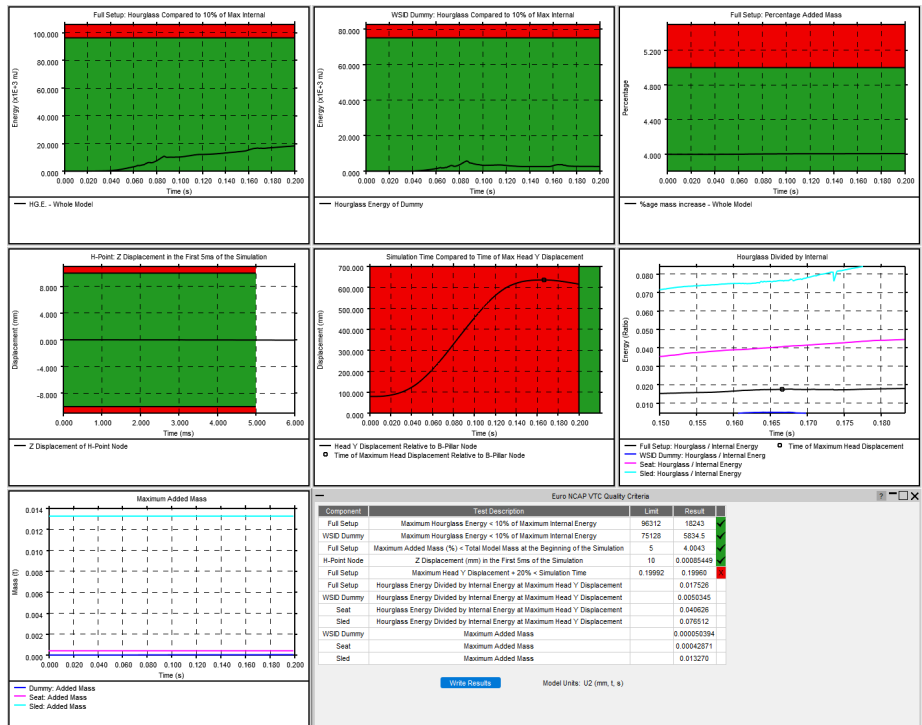
Fig.4: Euro NCAP VTC Quality Criteria workflow in Oasys T/HIS showing graphs of processed LS-DYNA results data.
