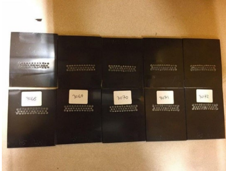
Fig.10: Sonic weld in coupons after test
