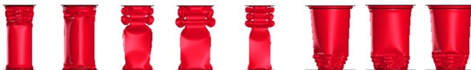
Fig 3: Different geometries of the Tube Crush model.
