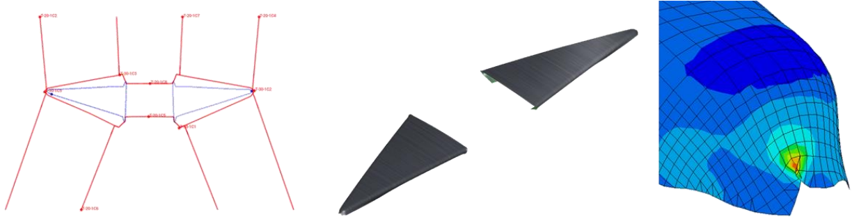
Figure 7 Left: Trimming curves (red) and target contours (blue). Middle: Final part after all forming operations with the initial trimming curves. Right: Wrinkling of the material at the corner of the part after the first iteration without using segmented trim line development. Mesh and thickness contour plot
