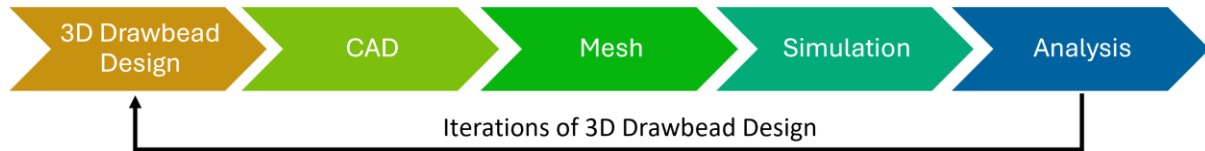
Fig.1: Drawbead design cycle with 3D geometric bead.
