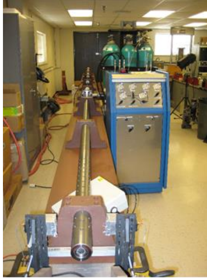
Fig.2: Tensile SHPB in the SwRI Engineering Dynamics Department.
