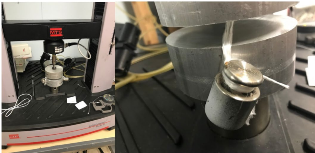
Figure 4: Compression tests of tow bundles.
