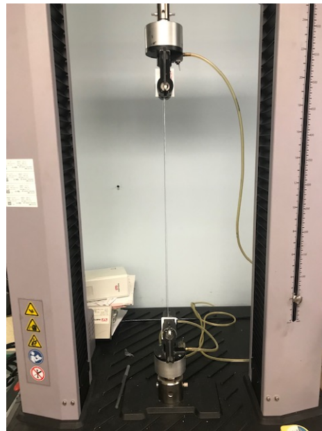
Figure 3: Tensile test of a single tow.
