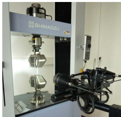
Figure 1: Tensile testing equipment and optical measurement system by GOM ARAMIS.
