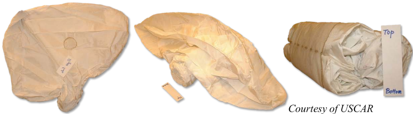
Fig.6: Photos of the PAB from USCAR research in unfolded, partly-folded and folded states
