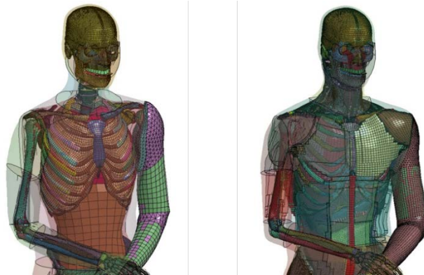
Figure 1. FE model comparison between simplified (left) [9] and detailed (right) models
