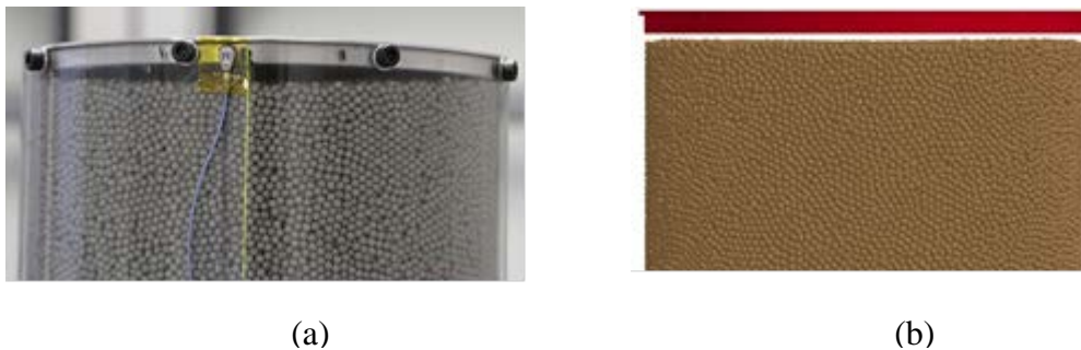
Fig.11: Illustration of the settling phenomenon occurring during the tank oscillations ((a) experimentally and (b) numerically)
