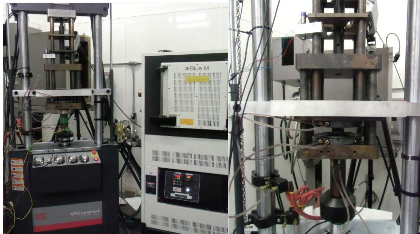
Figure 10. Example of a hot stamping apparatus used for validation
