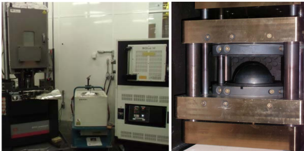
Figure 4. High temperature Nakazima setup
