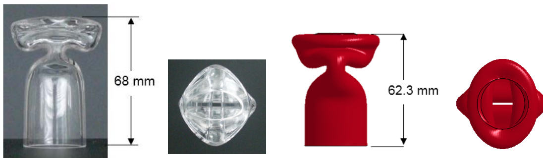
Figure 21 Deformed shape after buckling (Left: Experiment, Right: Simulation)
