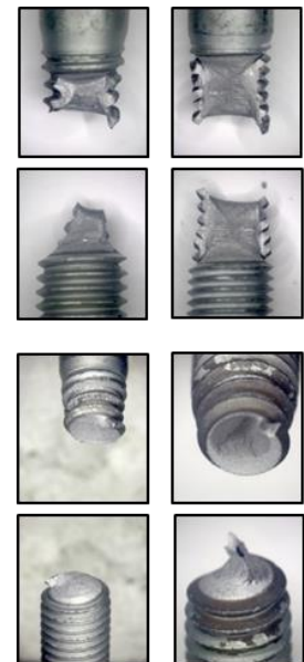
Figure 5: Different crack pattern in the thread under tensile loading
