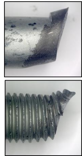
Figure 9: Fracture characteristics under combined load in the shank (top) and in the thread (bottom)
