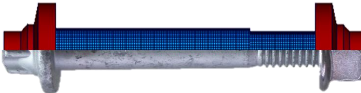
Figure 11: The detailed bolt model compared to the real bolt
