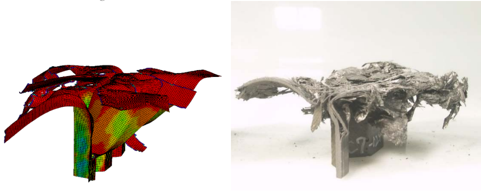
Figure 13: Comparison of simulation and tests for the corrugated double thickness 0 degree crush.
