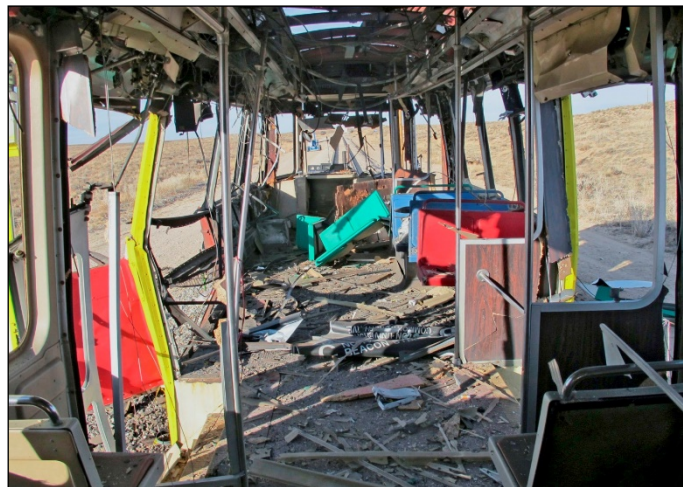
Figure 16 - Interior of the light rail car after internal charge test
