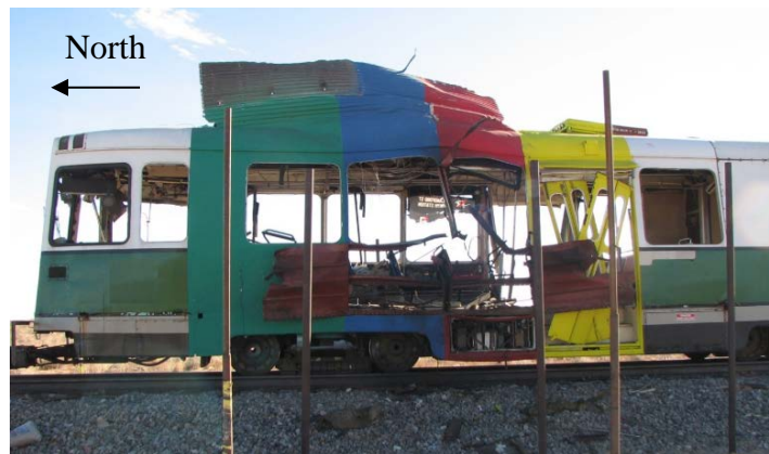
Figure 15 - Exterior of the light rail car after internal charge test
