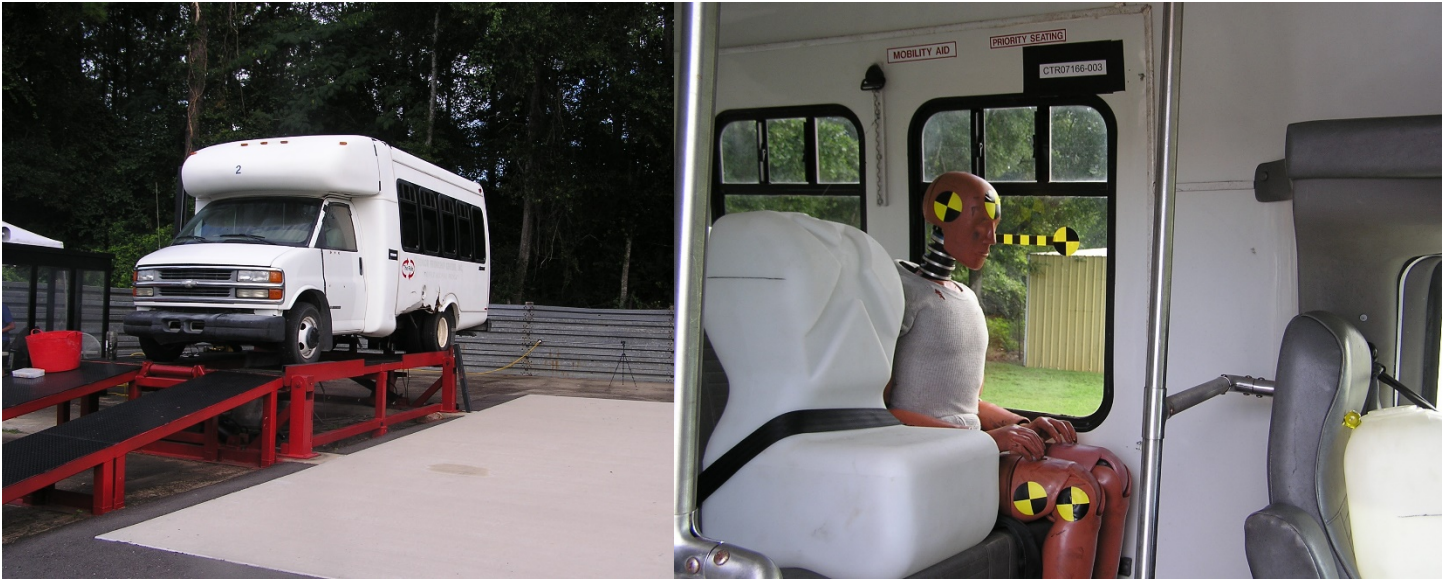
Fig. 1 Tilt table test according to Florida Standards and ATD's position.
