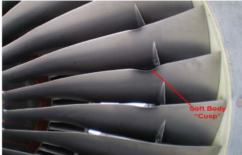
FIG. 1: Picture of typical fan blade damage due to bird-strike [1]
