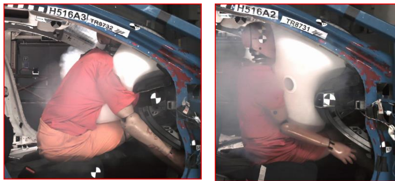
Figure 12, Depowered first stage inflator in ub50%-ile and ub5%-ile sled test
