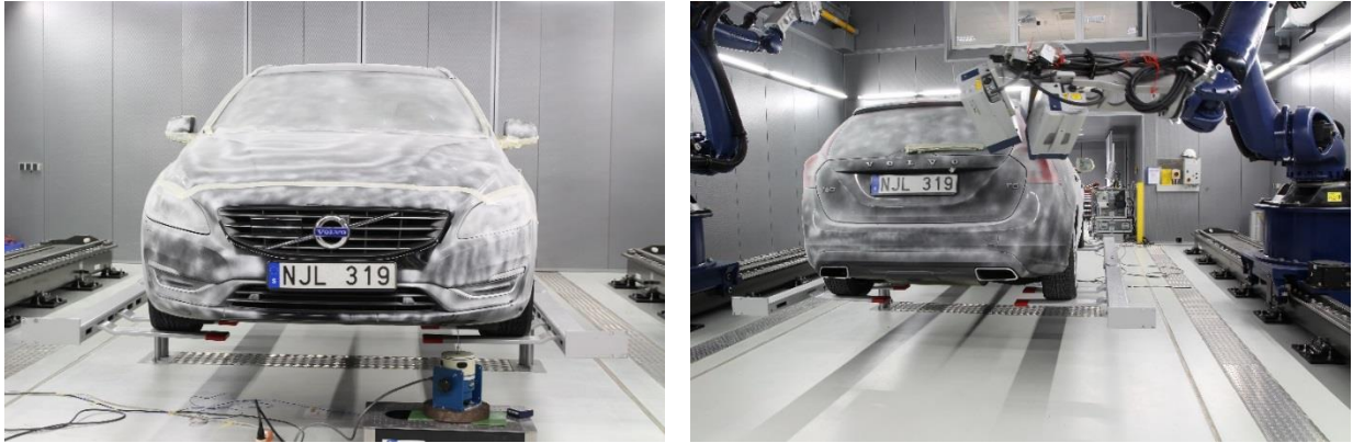
Figure 5. Measurement of Relative Displacement using the RoboVib from Polytech
