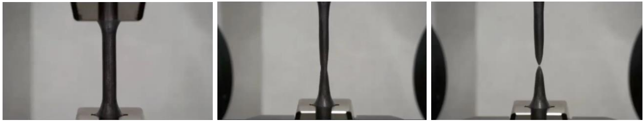
Fig.4 Deformation of specimen in tensile test
