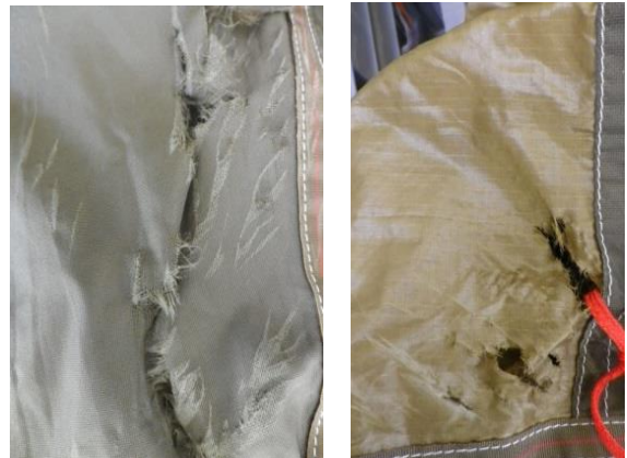
Figure 1 : Example of tears seen on parachute structures.
