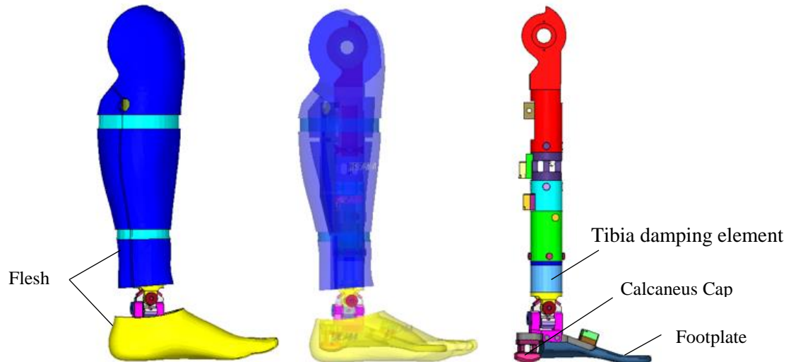
Figure 1. The WIAMan-LX which includes all components from the knee clevis to the foot. Shown here both fleshed (left) and defleshed (right)
