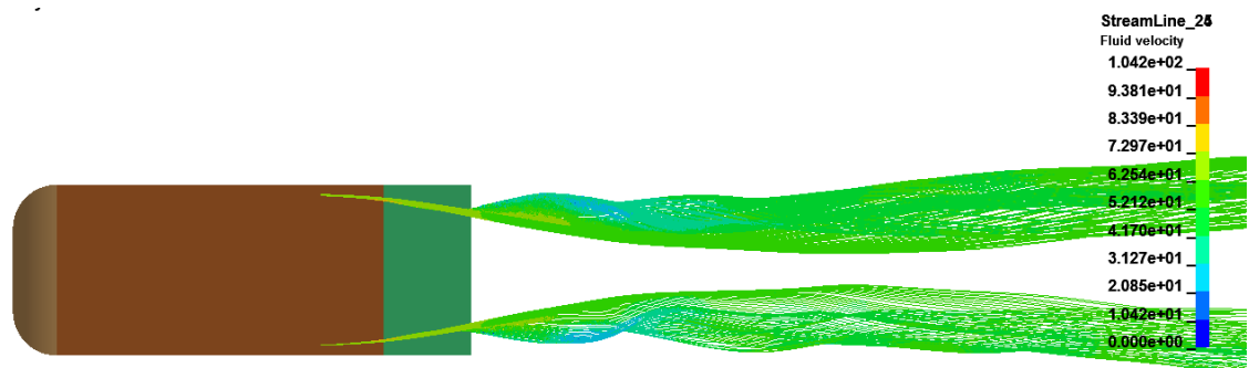
Figure 9: Development of the counter-rotating trailing vortex system within the wake of the 25° slant Ahmed body. Average fluid vector visualization at different locations in the wake of the body ( x = 0 ), a) x = 0.01 , b) x = 0.08 , c) x = 0.2 , d) x = 0.8
