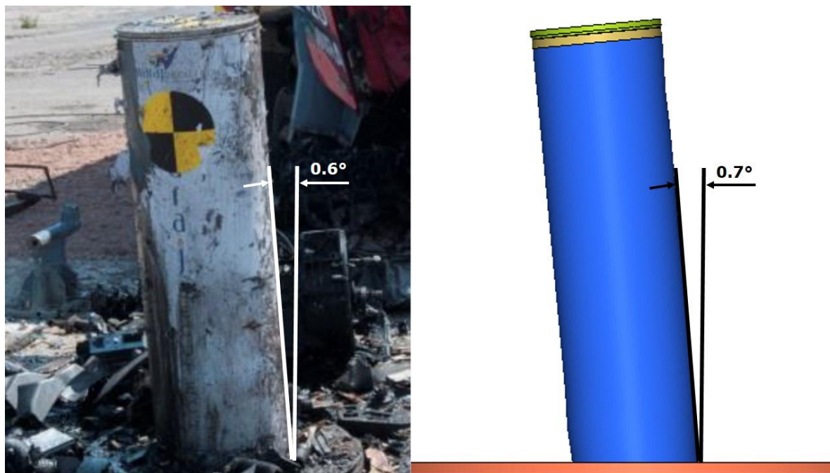
Figure 8 – Comparison of Bollard Angular Deformation between Physical Test (L) and FE Simulation (R)
