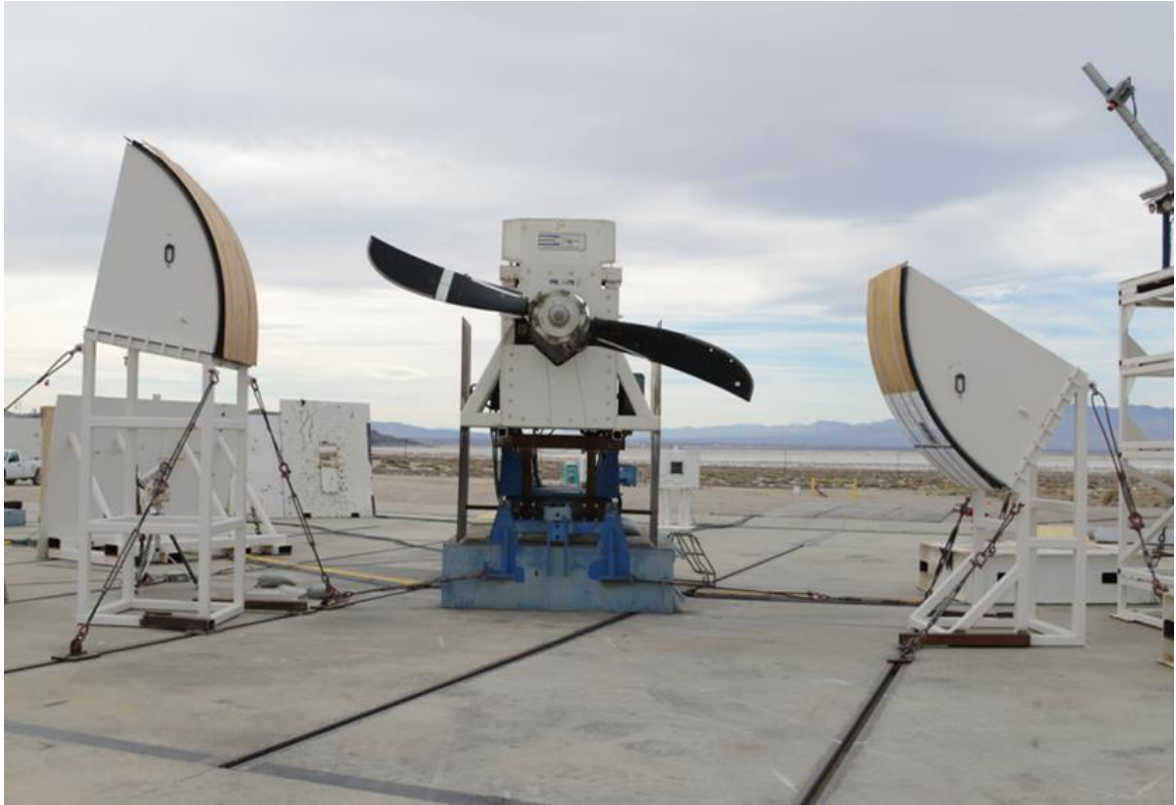
Figure 6. Blades mounted on the spin fixture. Test panels are shown on either side of the fixture.
