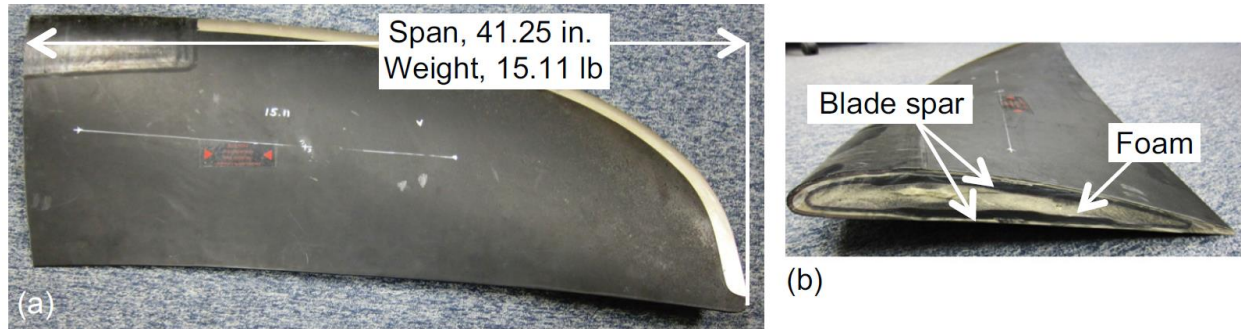
Figure 2. Outer section of blade used for analysis and full scale testing. (a) Section length and weight. (b) Blade cross section.
