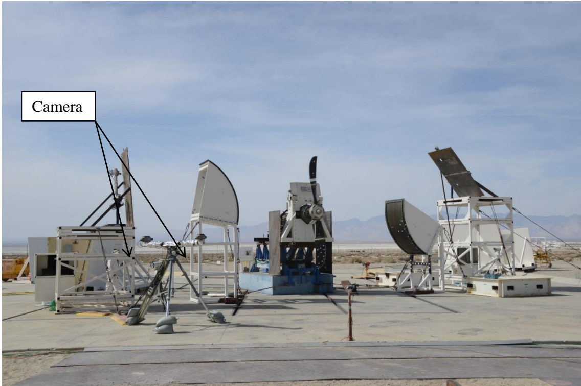
Figure 8. Cameras used for Measuring Blade Kinematics
