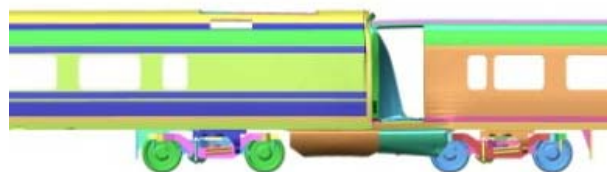
(b) Interface between back of power car and first passenger carriage
