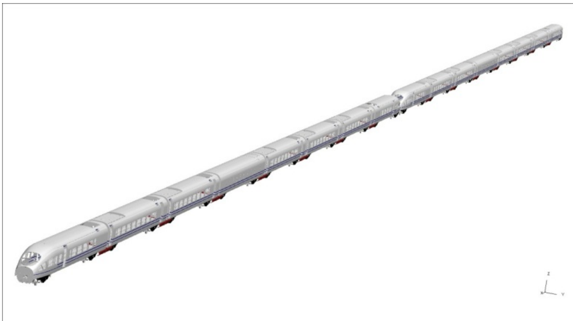
Figure 9 – Detailed CRH380 Model for LS-DYNA crash simulation
