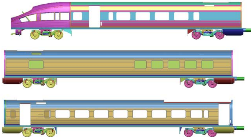
Figure 8 - Carriage models - From top to bottom: Motor, Restaurant and Passenger cars)
