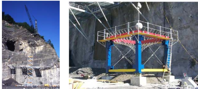
Figure 2: The specifically-built test rig for rock fall tests (after Volkwein, 2004)
