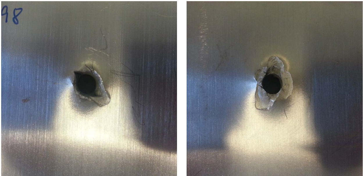
Figure 5. Hole from 7.62 mm armour-piercing projectile in 20 mm thick target plate. Left: front side of plate where projectile enters. Right: Back side of plate where projectile leaves.
