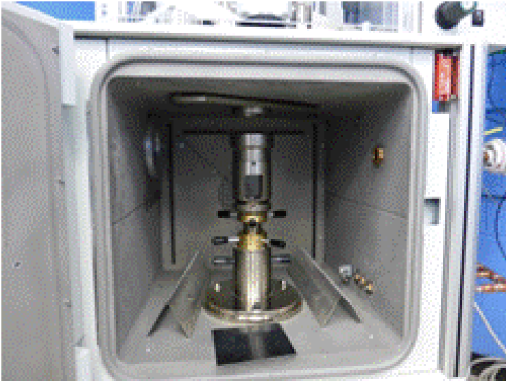
Figure 8: Drop Tower Plaque Impact Testing
