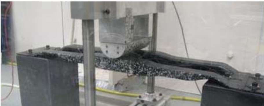
Figure 9: Drop Tower Beam Impact Test
