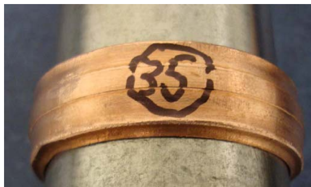
Figure 9. Copper Ring Sample Joined to Steel Bars at 45-KJ
