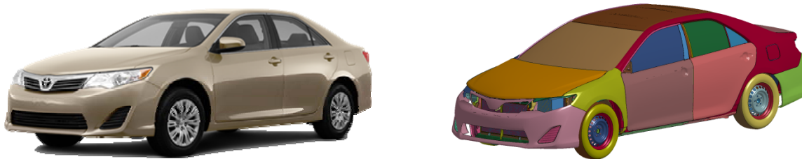
Figure 1 – Actual Vehicle and FE Model of a 2012 Toyota Camry Sedan
