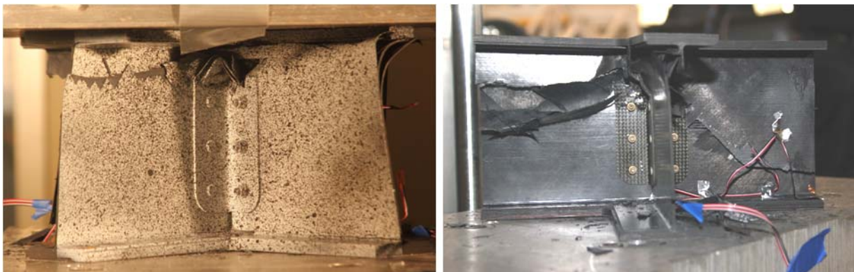
Figure 13. Post-test images of cruciform specimen following the 8-ft drop test.
