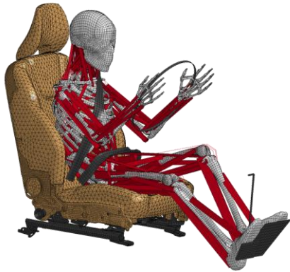
Fig.3: SAFER Active HBM in a driver braking simulation [2].
