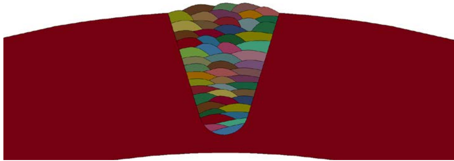
Fig. 11: Cross section with 53 passes SAW
