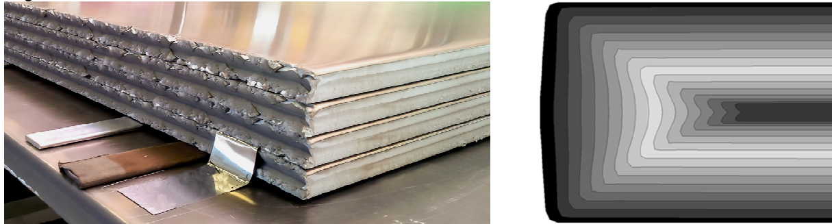
Fig.9: Real billet edge cracks (right) and calculated edge deformation (left) of 5xxx series aluminium alloy after hot rolling at the new hot rolling mill using bigger billet dimensions
