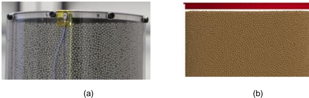
Fig.14: Illustration of the settling phenomenon occurring during the tank oscillations ((a) experimentally and (b) numerically)
