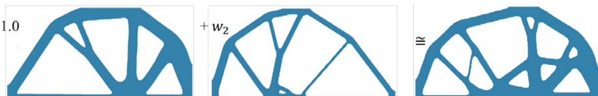
Fig.2: Multi-point method. Final topology depends on load case weights, hence load case weights can be used as global parameters.
