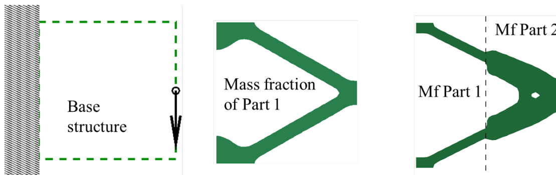
Fig.1: Multi-point method. Final topology depends on part mass fractions, hence part mass fractions can be used as global parameters.
