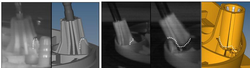
Fig.6: Experiment Bosch Impact Test – estimation of the 2 parameters *MAT_ADD_EROSION card
