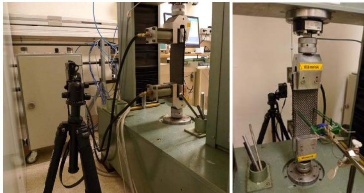
Fig.2: Experimental setup used for the tensile tests
