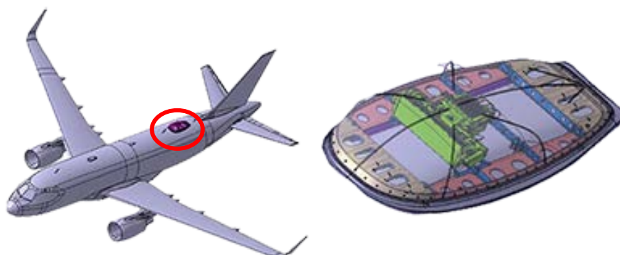
Fig.1: Antenna, radome and interface structure
