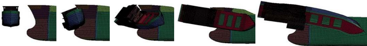
(b) collision behavior by striking ship with bulbous bow
