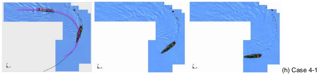
Fig.23: Full-scale rapid turning simulation behavior according to scenario in top view
